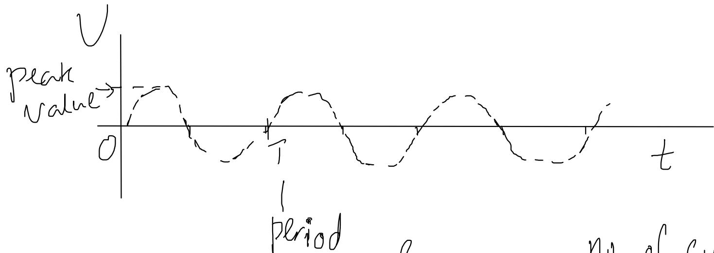
$$\text{frequency} = \frac{\text{no. of cycles}}{\text{per unit time}}$$
