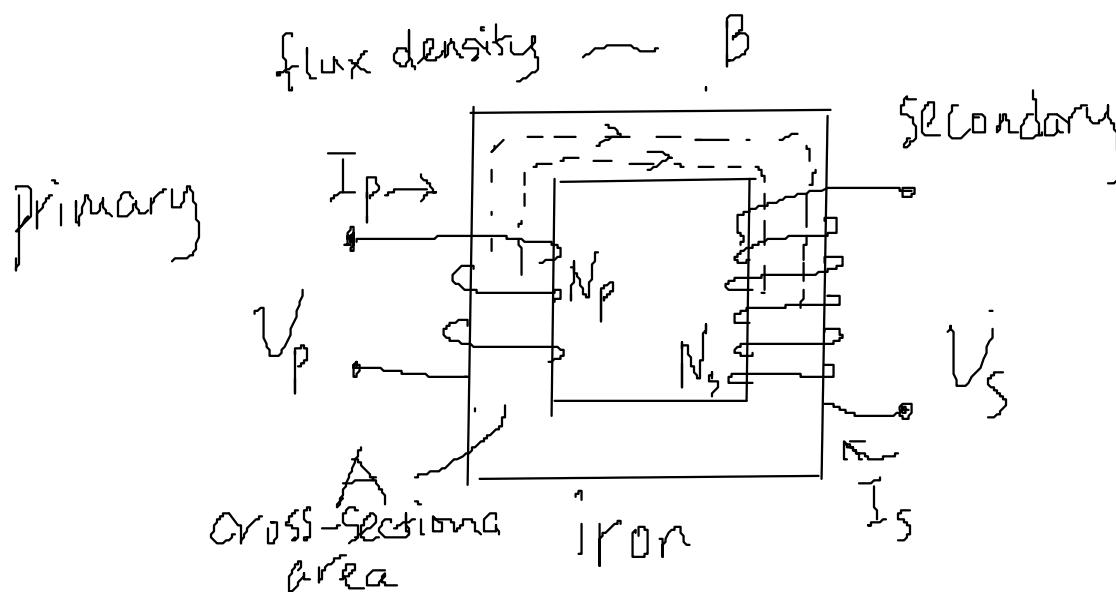
Flux thru' both primary and secondary coil
